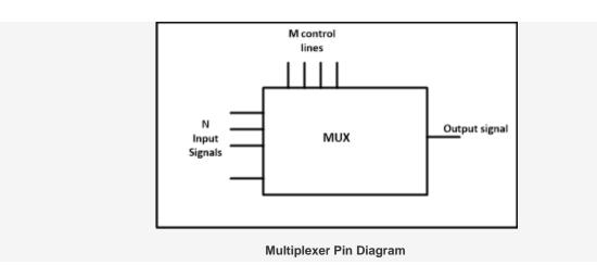
Following figure shows the general idea of a multiplexer with n input signal, m control signals and one output signal.
