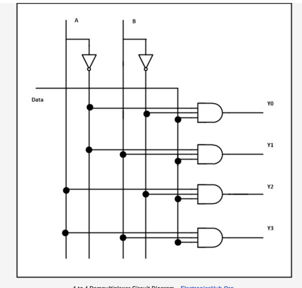
1 to 4 Dempultiplexer Circuit Diagram – ElectronicsHub.Org
