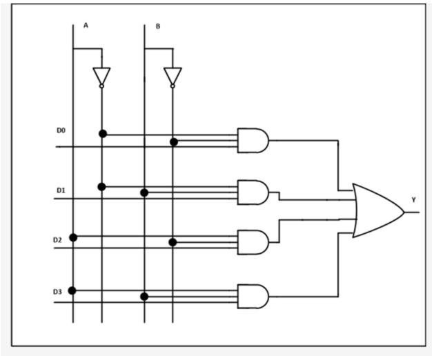
4 to 1 Multiplexer Circuit Diagram – ElectronicsHub.Org
