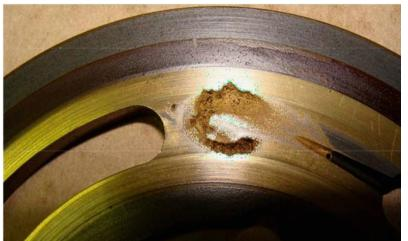
• Damage (erosion) due to cavitation on a marine propeller.
