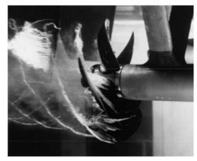
• Bubble formation due to high velocity (flow-induced boiling).
