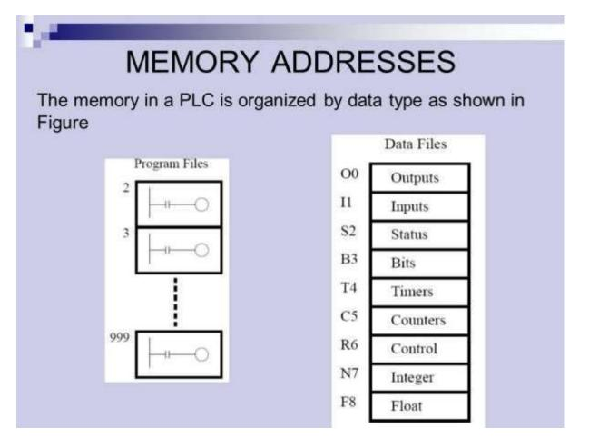
**Output image status bit:** This file store the status of discrete output terminals .during program scan, this data is updated and at the end of program scan, It is transferred to real world outputs.
