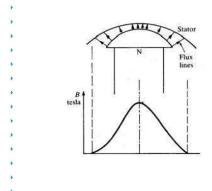
Non-linear variation in flux across pole face produces sinusoidal change in the induced EMF
