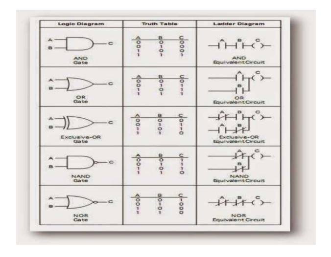
**OR Combination:** For logical 'OR' combination of two or more inputs are put in parallel to each other. The rung condition will be TRUE if any one of the input is true if the inputs are false then only the rung condition will be false.
