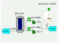
Typical SCADA mimic shown as an animation. For process plant, these are based upon the piping and instrumentation diagram.
