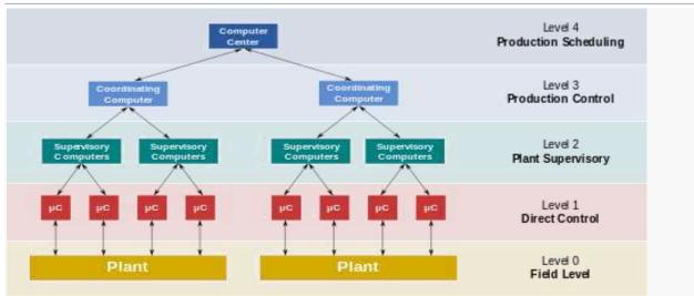
The SCADA concept in control operations.
