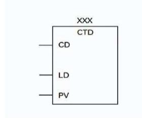
Each time the input CD turns ON the counter decrement one from the preset value. Whenever LD (load) input becomes high then the preset value is reloaded to the counter from the current value.
