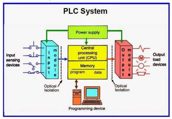
The basic parts of PLC architecture are:
