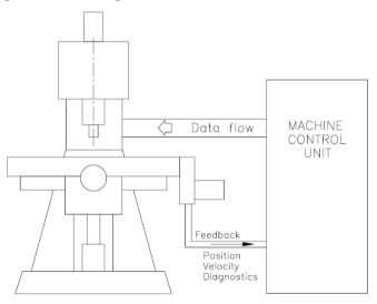
Figure 3.1 : Computer Numerical Control (CNC) Machine
