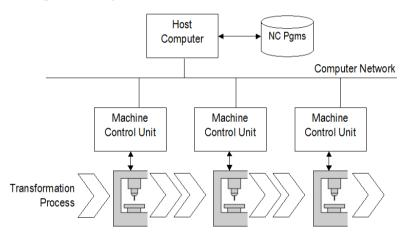
Figure 3.3 : Direct Numerical Control (DNC) Machine
