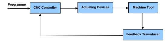
Figure 3.2 : Computer Numerical Control (CNC) System
