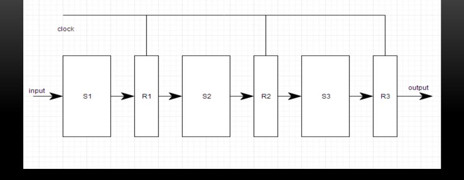
Pipeline system is like the modern day assembly line setup in factories. For example in a car manufacturing industry, huge assembly lines are setup and at each point, there are robotic arms to perform a certain task, and then the car moves on ahead to the next arm.
