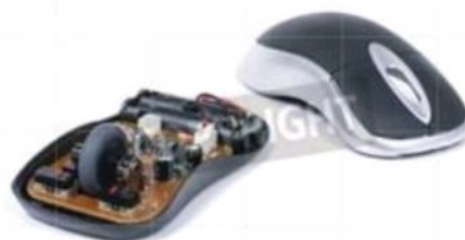
▲ Figure 1.1 The inside of an optical mouse
