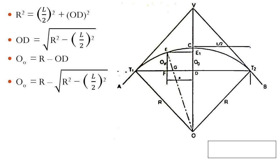
In order to calculate ordinate Ox to any point E, draw the line EE<sub>1</sub>, parallel to the long chord T<sub>1</sub> T<sub>2</sub>. joint EO to cut long chord in G.
